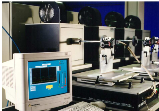
This five-station system runs a variety of tests on windshield wiper motors and window regulators, while increasing reporting, logging and analyzing opportunities.
